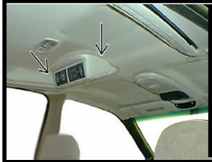
Remove and **FIGURE** ontrols from console and lay them in a safe place. Discard console. See Fig. 2.
